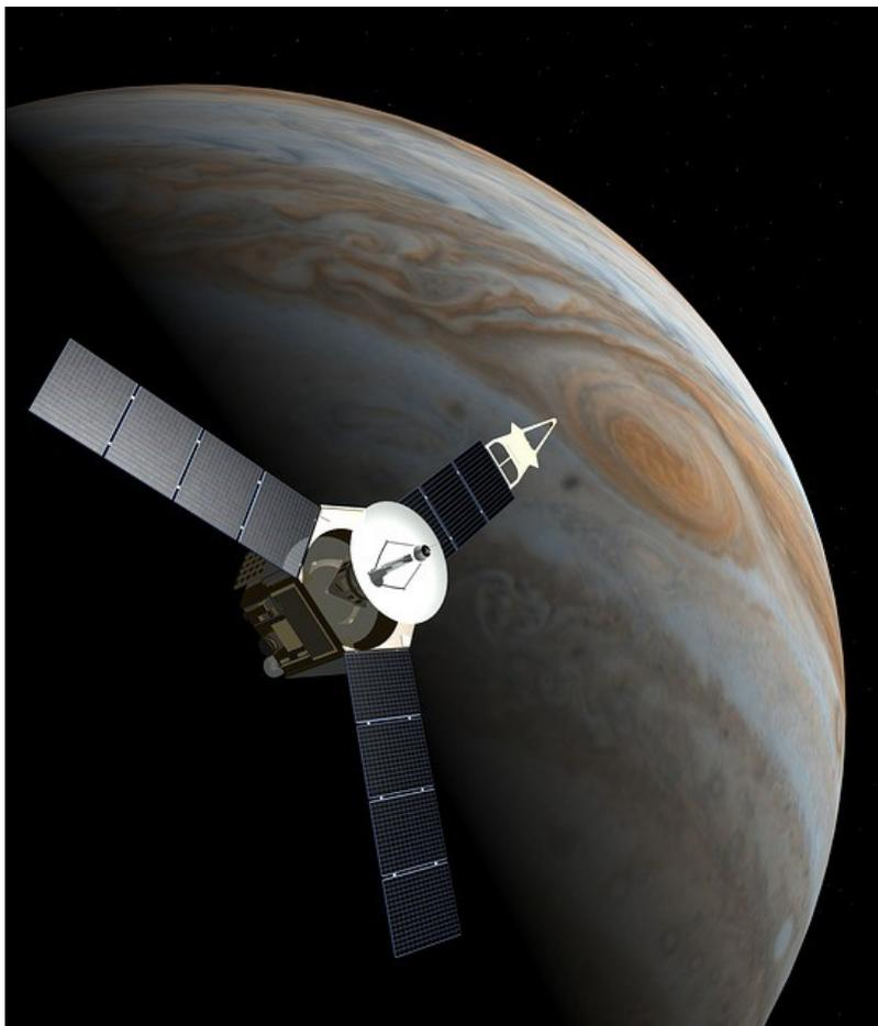
There are many instruments on the Juno. The JUNOCAM captures images sent back to earth. The JIRAM visualizes the Aurora and clouds in the infrared range. The UVS also visualize the auroras but in the ultraviolet range. The WAVES studies the magnetic field. JADE and JEDI are studying the particles that interacts with the magnetic field and the auroras. Gravity Science and Microwave Radiometer will provide the interior structure of the planet, while
