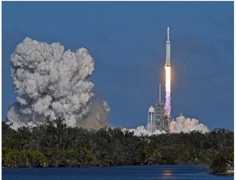
Falcon Heavy is the most powerful operational rocket in the world. It can lift into orbit nearly 64 metric tons (141,000 lb.). Falcon Heavy is able to
